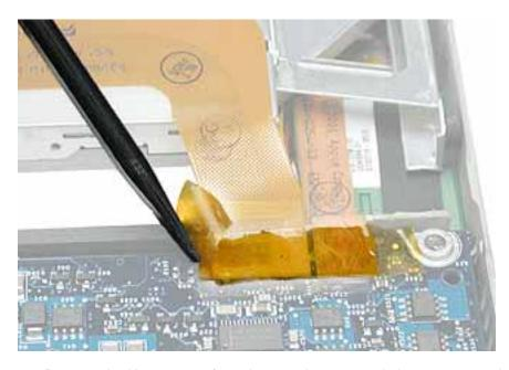
12. Remove the Kapton tape from the two-pin power switch connector at the right corner of the logic board. Disconnect the two-pin connector.
