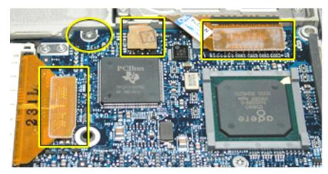
9. Remove the two identical Torx T8 screws and their washers, located near the center of the board.
