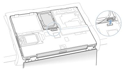
2. With a Torx T8 screwdriver, remove the two screws **(Figure 9)** that secure the hard drive to the mounting bracket and then gently remove the hard drive.
