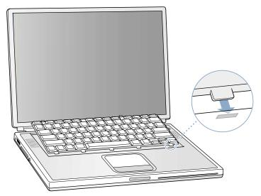
3. Lay the keyboard flat into the keyboard opening.
