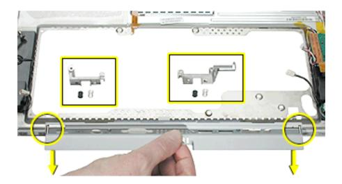
3. Remove the L-shaped pin from each end of the I/O door.
