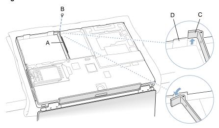
3. Verify that the replacement hard drive has four screws (Figure 11A), two on each side, with four rubber stoppers (Figure 11B) attached.
