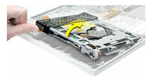
**Note:** There are four rubber stoppers (two on each side) on the DVD-ROM drive that fit over screws. Remove any that may have fallen off inside the computer.
