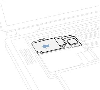
3. Line up the hexnut screw hole, in the left front corner of the modem, with the hole in the logic board. The modem should lie flat.
