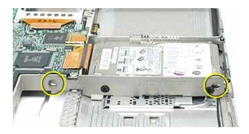
**Important:** Verify that the DVD-ROM drive cable does not get caught on the rib frame as the drive is lowered into place. When the rubber stoppers are inserted, push down on the side. Press at all four corners of the drive to verify that it rests flat and is secure.
