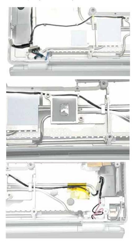
18. Install the replacement rib frame and/or heat exchanger, and reassemble and test the computer.
