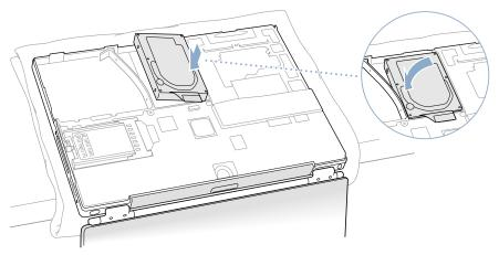
5. Lift the mounting bracket (Figure 13A) over the battery bay tab and lower it to its original position. Line up the rubber stoppers on the hard drive until they fully seat into the holes in the bracket.
