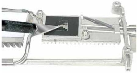
21. On the replacement logic board, center new thermal transfer material over the epoxy cap on the microprocessor chip. Press it into place.
