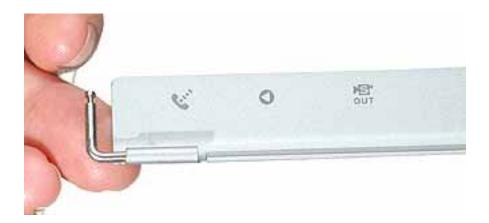
4. When installing the replacement I/O door, make sure each L-shaped pin threads through the top case, inner clutch mount, spring, and plug.
