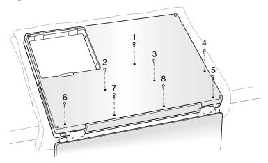
**Note:** The following three steps explain how to remove the bottom case by disengaging it at the left and right sides and then carefully pivoting it forward.
