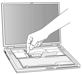
12. Locate the keyboard cable connector. (Figure 6)
