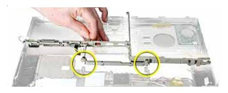
14. Disconnect the audio cable at each end of the heat exchanger.
