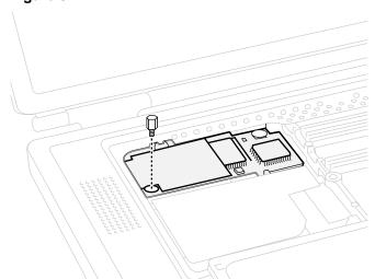
2. Pull up on the right, front corner of the modem to disconnect it from the logic board. (Figure 7)
