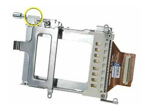
4. When installing the replacement PC card cage, ensure that the metal flange that is closest to the PC card eject button goes underneath the rib frame and metal liner at the battery latch.
