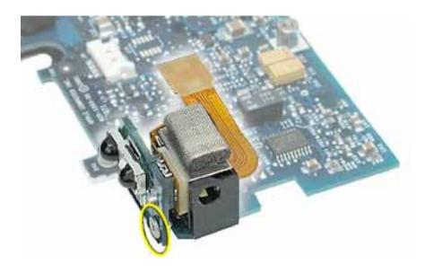
16. Remove the infrared communications board for installation on the replacement logic board.
