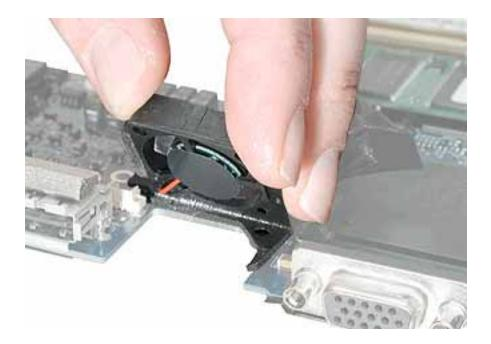
4. When installing the replacement fan, first use a black stick to push the cone-shaped rubber pin into the hole on the logic board. (If necessary, use needlenose pliers to pull the rubber pin through to the other side of the logic board.) Then, peel away the protective cover from the adhesive that lines the three sides of the fan. Align the fan over the logic board opening and press the fan into place.
