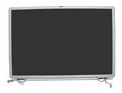
6. **Important:** When the replacement display module is installed, and before the clutch covers are installed, test that the display is seated properly. With the computer upright and closed, press the computer latch. The display module should pop up slightly if the module is properly seated.
