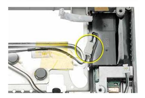
15. Pivot the heat exchanger out of the top case assembly. Be careful where it might catch at the LVDS cable.
