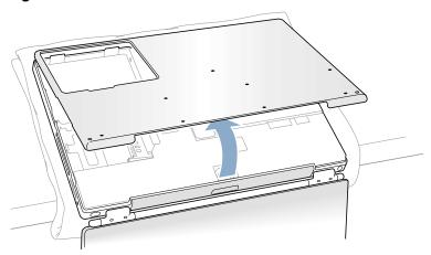
11. Touch the computer's inside framework (a dull gray conductive composite material) to discharge any static electricity, as shown. (Figure 7)
