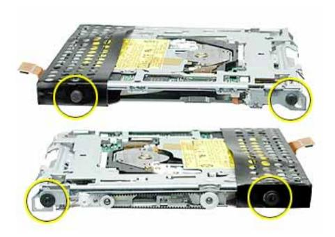
When installing the replacement drive, first insert the stoppers on the inner side of the drive into the openings on the rib frame. Then while holding the inner side of the drive in place, carefully guide the rubber stoppers on the outer side of the drive past the edge of the rib frame.
