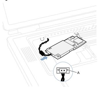
2. Carefully guide the cable into the space under the edge of the keyboard opening and lay the modem into the modem opening (Figure 11).
