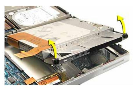
**Note:** There are four rubber stoppers (two on each side) on the DVD-ROM drive that fit over metal posts at the corners of the drive. Remove any that may have fallen off inside the computer.
