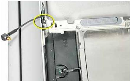
13. Lift the rib frame off of the heat exchanger. If the heat exchanger sticks to the rib frame, press gently on the heat exchanger near the two connection points shown.
