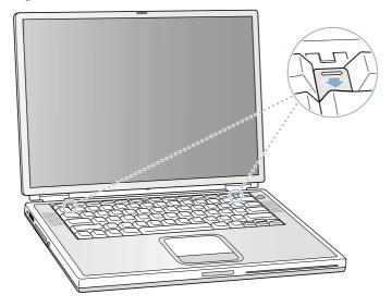
5. Release the tabs to secure the keyboard in place.
