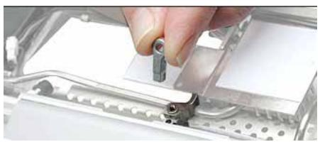
12. Remove the four identical black screws from the rib frame. (You might need to move aside the AirPort antenna cable to reach one of the screws.)
