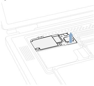
3. Pull the modem up and to the right slightly to reveal the modem connector cable attached to the left end of the modem. (Figure 8)
