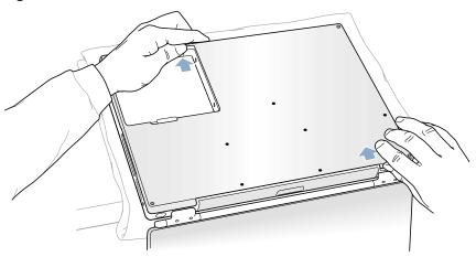
10. When both sides have released, lift up on the edge of the bottom case that is closest to you; carefully and evenly pivot it over the front edge of the computer until it releases. (Figure 6)
