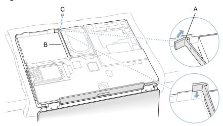
7. Connect the hard drive cable connector (Figure 14) to the logic board.
