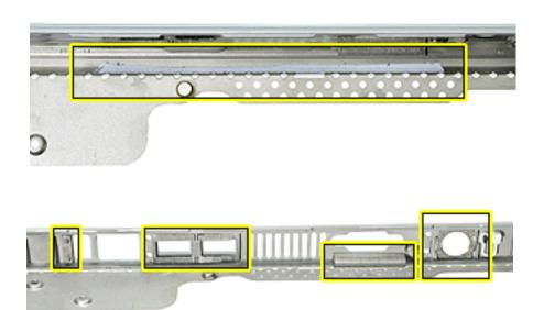
5. **Important:** Make sure you transfer the backup battery cable from the original top case to the replacement top case. The backup battery cable adheres to the inner top case with two pieces of tape, and is routed as shown.
