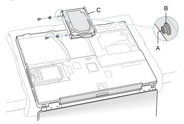
4. Insert the right side of the drive first, until the rubber stoppers fit securely into the holes in the bracket, and then insert the left side of the drive. (Figure 12)
