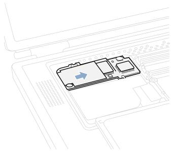
4. Carefully disconnect the modem cable connector (Figure 9) and remove the modem from the computer.
