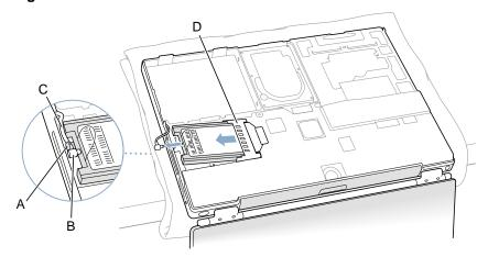
**Important:** If the AirPort Card is not being replaced right away, replace the antenna cable connector into its holder **(Figure 10B)** and pull the loop of the antenna cable up slightly and away from the edge of the computer case. This prevents the cable from interfering with the PC card slot, below, or getting pinched during reassembly.
