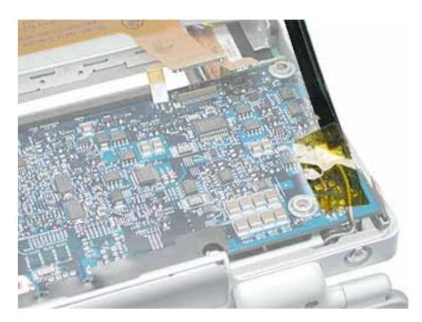
13. Grasp the logic board near the AirPort Card carrier. Gently tilt up the board, being careful where it catches on the back panel ports, integral mesh liner, and the disconnected cables.
