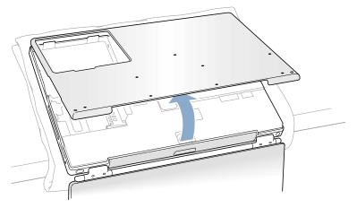
11. Touch the computer's inside framework (a dull gray conductive composite material) to discharge any static electricity, as shown. (Figure 7)
