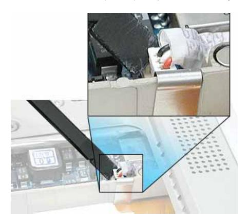
5. **Important:** With the bottom case removed, be careful when turning over the computer. Some components could become loose and fall out.
