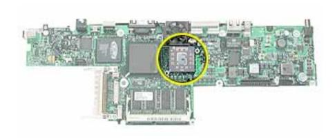
22. Install the replacement logic board, and reassemble and test the computer.
