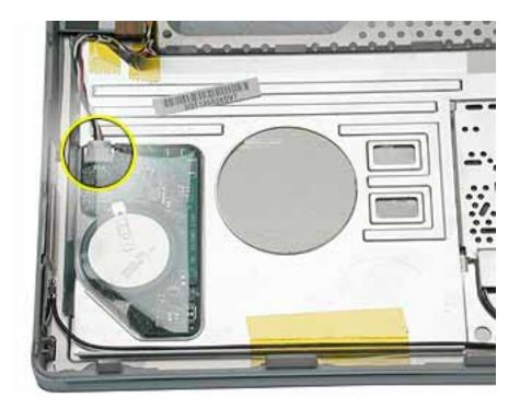
2. **Note:** The backup battery is compressed between two thin plastic sheets. The battery is held in place with adhesive on the lower plastic sheet.
