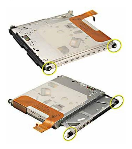
5. Warning: To prevent damage to the optical drive, handle the drive only by the corners. Do not press on the body of the drive.
