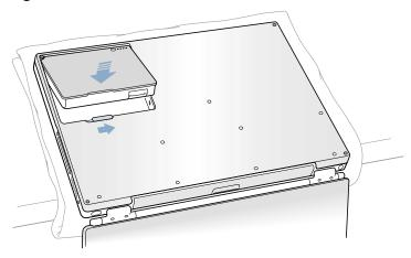
6. Turn the computer over so that the optical drive slot faces you. Verify that the bottom case is flush with the front edge of the slot. If the case is slightly bowed and there is a gap near the center of the slot, carefully pull the bottom edge of the slot until it clicks into place and becomes flush with the bottom case. (Figure 15)
