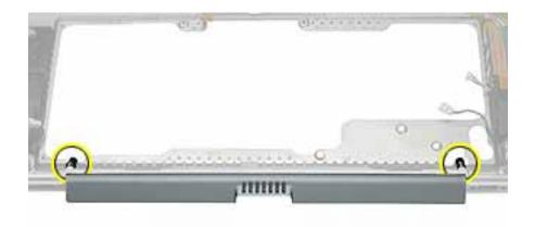
2. Lift off the inner clutch mounts, and pull door away from the top case.
