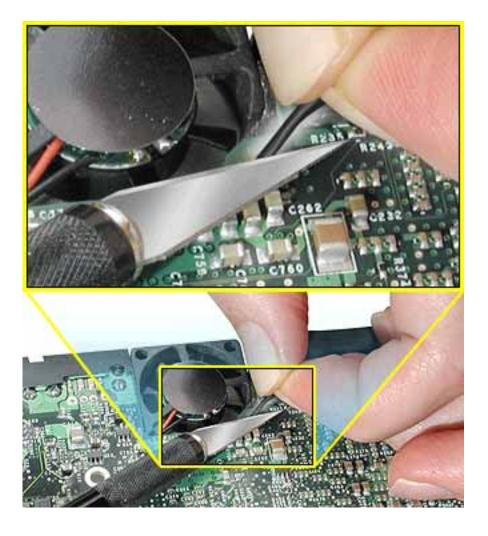
3. Turn over the logic board, and tilt up the fan to remove it completely from the logic board.
