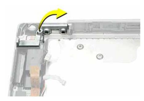
2. Tilt up the inverter board to lift it off of the top case.
