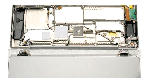
10. Open the I/O door, and remove the four identical Torx T6 screws.
