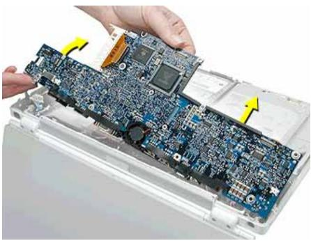
**Note:** When reassembling the computer, make sure the replacement logic board ports align completely with the openings in the back panel.
