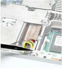
**Note:** When reassembling the computer, tuck down the battery cables so they do not get in the way when the keyboard is installed.
